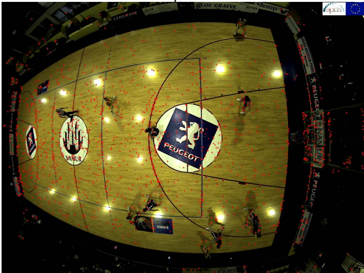
Figure 8-Result of the SIFT performed on fisheye images, where each red cross represents a final key point.
