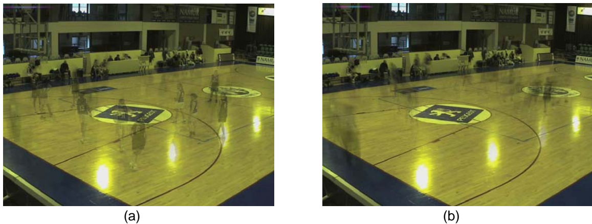
Figure 3-Effect of learning rate on the constructed background after 100 frames with (a) 10% (b) 50% learning rate
