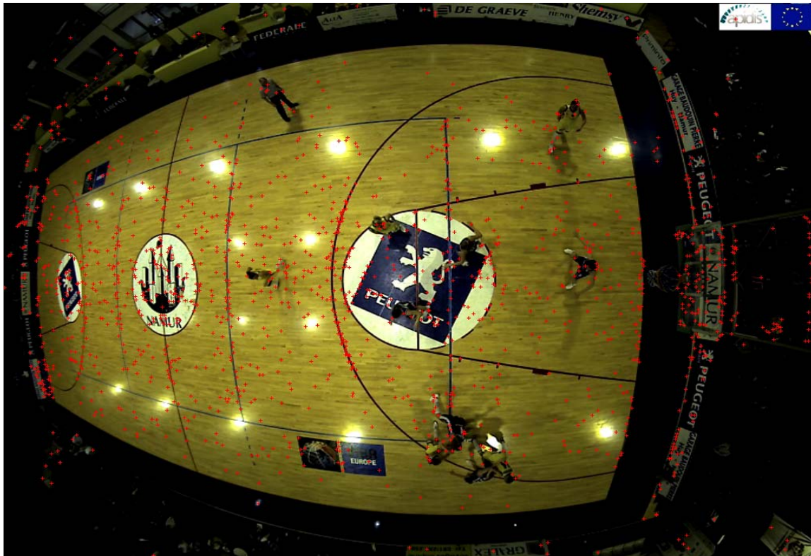
Figure 7-Result of the SIFT performed on fisheye images, where each red cross represents a final key point
