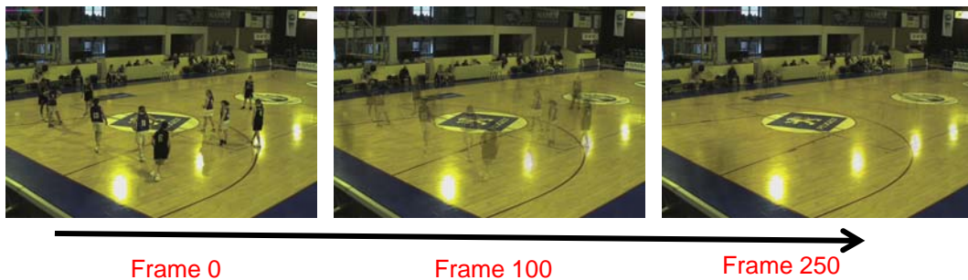
Figure 2- Results for background learning. Starting from frame 0, the foreground objects are removed from the image.
