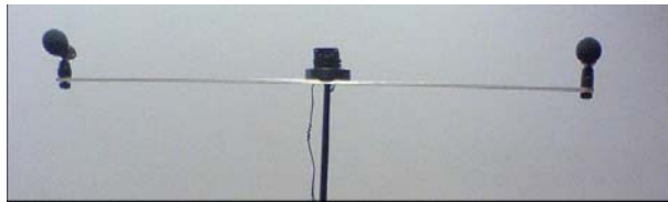
Figure 4: A STAC sensor consisting of a single camera and a pair of microphones in stereo configuration
